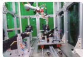
Screwing in lighting assemblies
