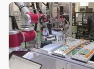
Screwing operations on lamp assembly
