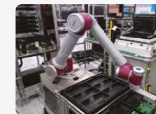
Gluing operations on PCs
